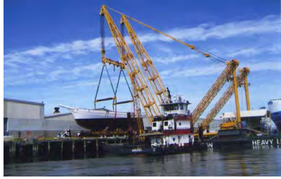
Figure 2-13: CMMC 500 ton Barge Crane Source: J. E. Oswald and Sons, 2009
