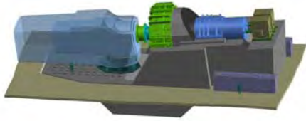
Figure 2-11: Wind Turbine Drivetrain Test Rig #1
