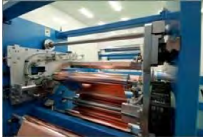
Coater Feed and Electrical Application
