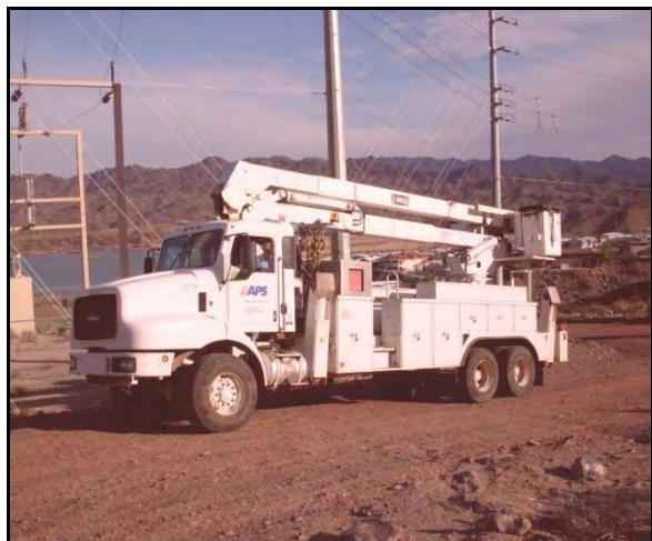
Photograph 2-7 Example of a Boom Truck
