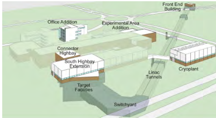
Figure 3–1. Potential FRIB Configuration: Straight Linear Accelerator Configuration Option
