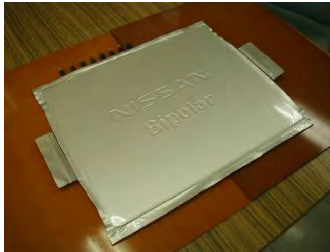
Figure 2.6. Single Laminated Battery Cell
