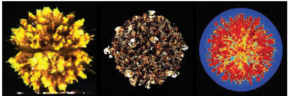
The attributes of a high explosive test (left) are closely predicted in a computer modeling capability (center) that produces a temperature map (right) of the hot matter and an eventual observed signature.
