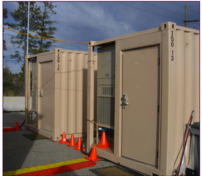
The radiography and nondestructive assay modules, or transportainers, of the MPF deployed at LANL during Operation Sputnik.
