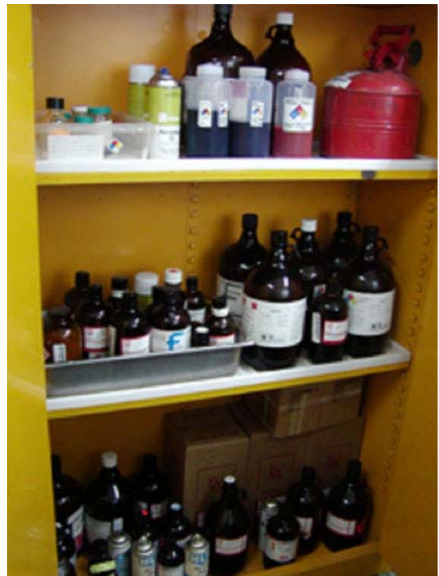
Legacy Waste in a Satellite Accumulation Area
