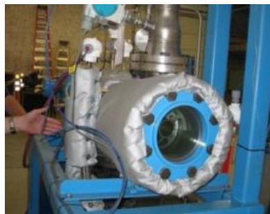
Pilot-Scale WFE, Vapor Discharge End
