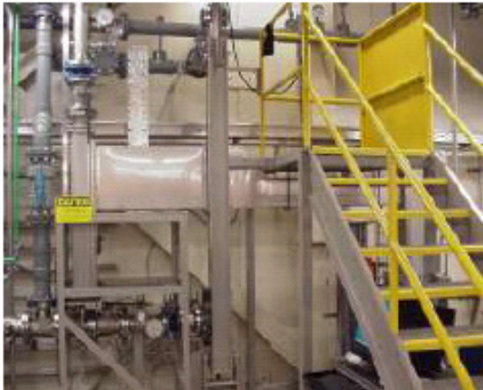
VISTA Loop 5x5 testing pressure drop & vibration
