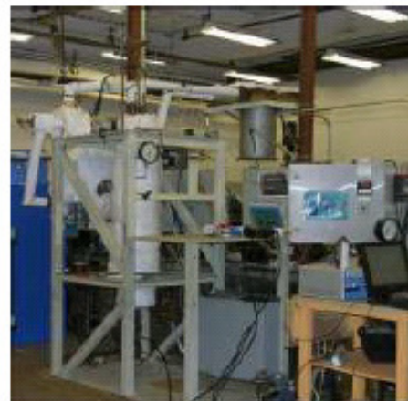
WALT Loop single rod CRUD and thermal testing
