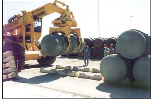
39 40 41 42 43 44 45 46 Figure 2-4 Stacking Depleted UF 6 Cylinders in a Storage Yard (DOE, undated a)
