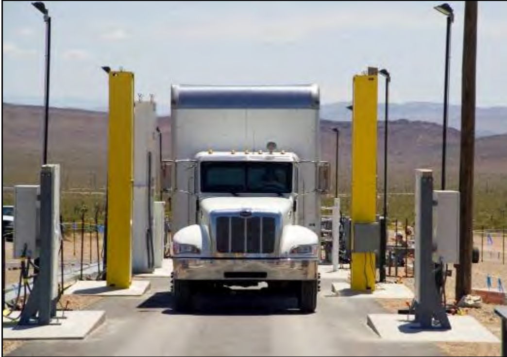
Figure 2-6 Radiological/Nuclear Countermeasures Test and Evaluation Complex Provides Capabilities for Evaluating Transportation Monitoring Equipment
