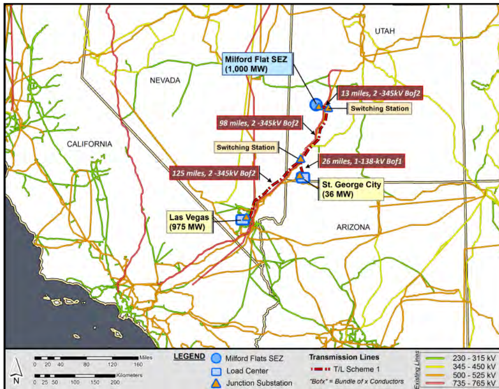
1 2 FIGURE 13.2.23.1-2 Transmission Scheme 1 for the Proposed Milford Flats 3 South SEZ (Source for background map: Platts 2011)
