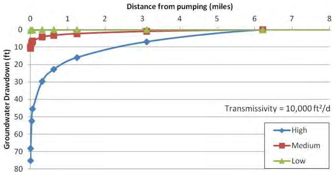
27 28 FIGURE 13.2.9.2-2 Estimated One-Dimensional Groundwater Drawdown Resulting from 29 High, Medium, and Low Groundwater Pumping Scenarios over the 20-Year Operational 30 Period at the Proposed Milford Flats South SEZ as Revised
