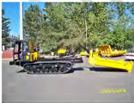
Morooka outfitted with a hook-lift showing an off loaded box. The chip box would be considerable larger than the box shown
