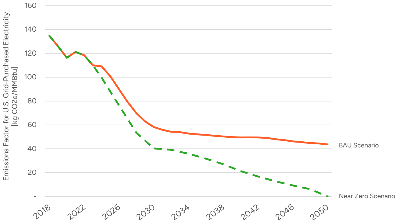
Figure B-1. Annual U.S. grid-purchased electricity emissions factors by scenario used for the Transformative Pathways modeling
