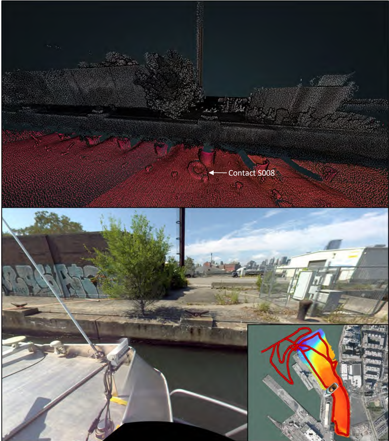
Figure 4. Vessel-based LiDAR draped with Bathymetry Point Cloud near Contact S008 (Tire)
