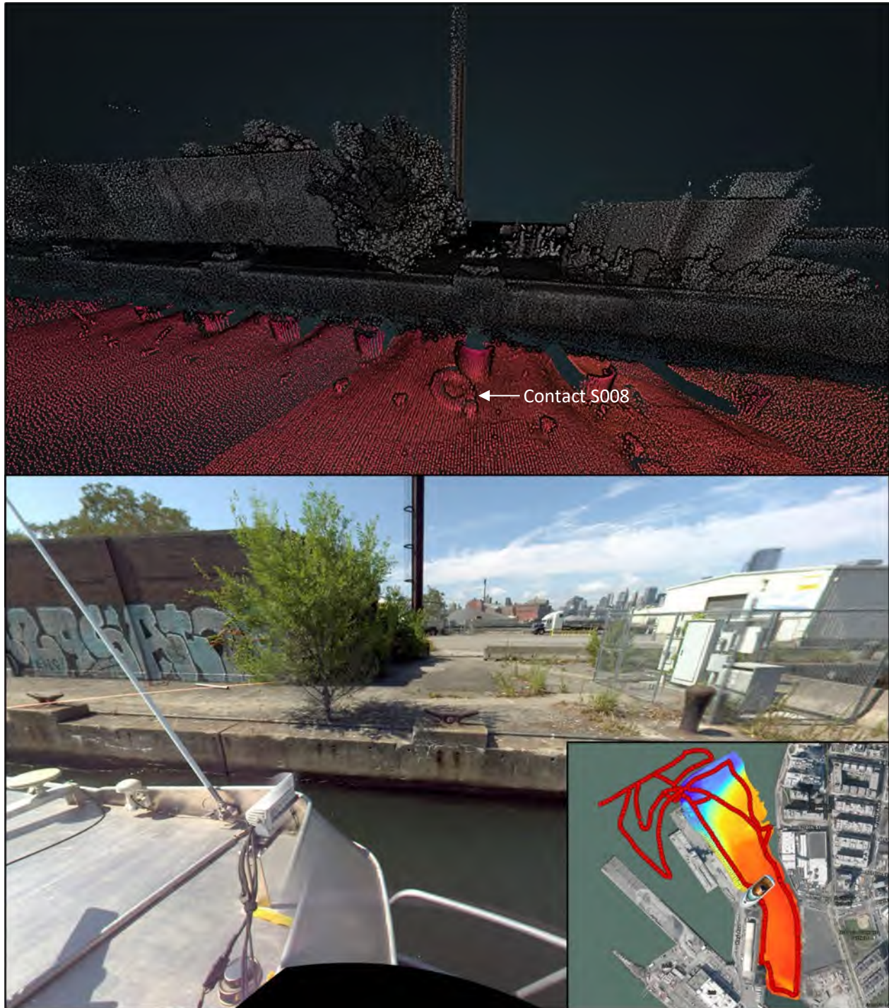
Figure 4. Vessel-based LiDAR draped with Bathymetry Point Cloud near Contact S008 (Tire)
