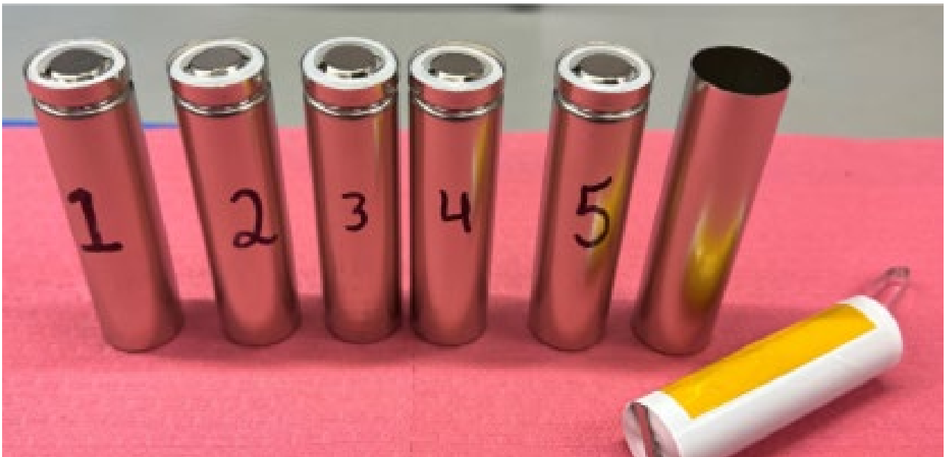
Figure 7. Li-Ion batteries in 18650 form factor with coal-based anodes
