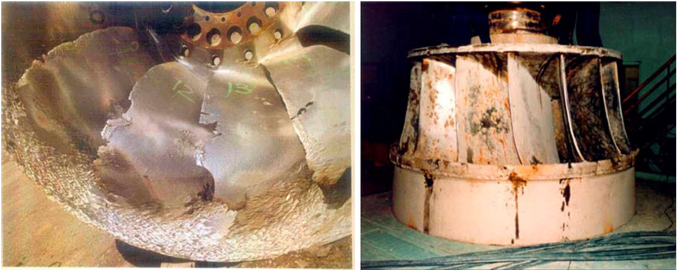
Figure 17. Examples of runner blades showing cavitation erosive failure. 221
