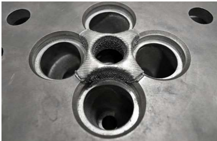
Figure 14. Repair of cast iron cylinder heads on heavy-duty engines by AM DED using high Ni containing alloy
