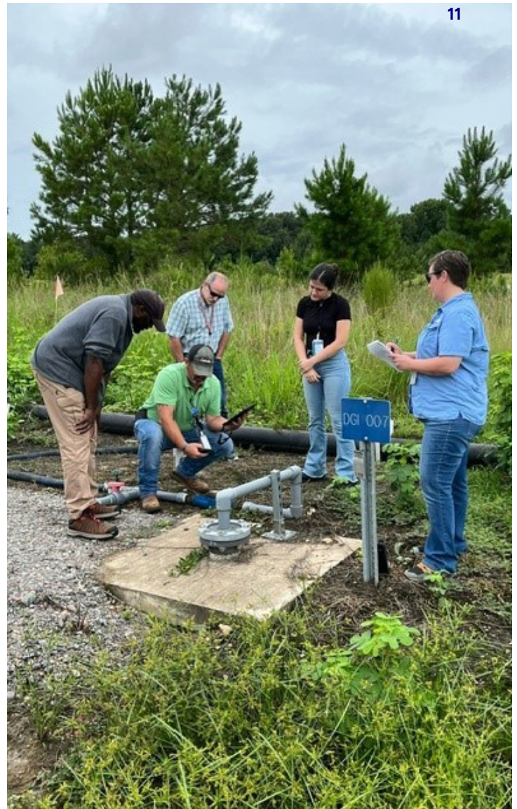
The D-Area Groundwater Treatability Study project team assesses artesian flow into an injection well onsite.
