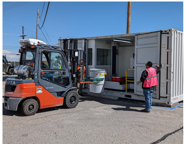
Waste Operations workers at TA- 54, Area G place a container of legacy TRU waste in the UDASS to analyze radioactive contents in waste drums.
