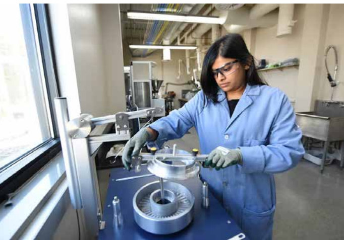
FCIC researcher Tiasha Bhattacharjee from INL testing ring shear equipment. Careful experimental work revealed variability in biomass mechanical attributes, important details for predicting the flow and comminution properties of biomass.
