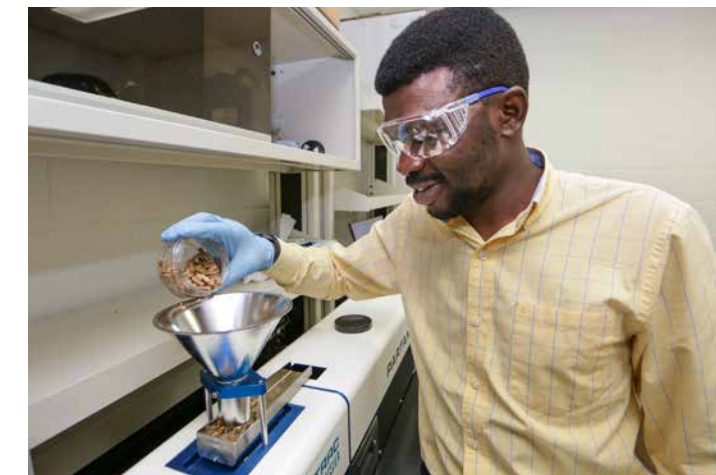
FCIC researcher Oluwafemi Oyedemi performing dynamic image characterization to assess particle size and shape distributions of woody biomass, which are critical material attributes for modeling thermochemical conversion processes.
