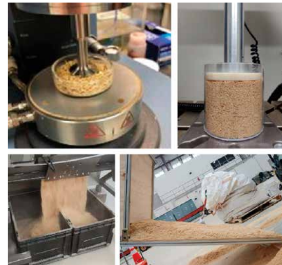
Figure 6. A variety of laboratory- and pilot-scale characterization tools were used to measure the physical and mechanical properties of biomass feedstocks under both static and dynamic conditions and to validate computational models of biomass flow. From left to right: Laboratory-scale rheometer, laboratory-scale uniaxial compression cell, pilot-scale adjustable wedge hopper discharge, and pilot-scale inclined plane flow tester.
