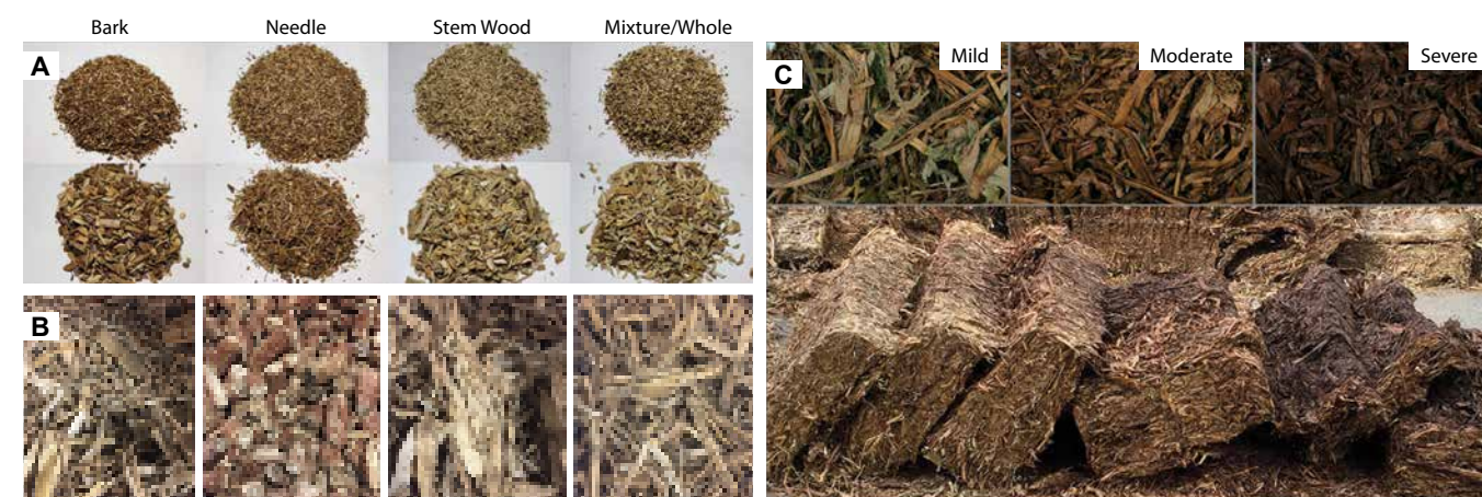
Figure 1. Feedstocks are intrinsically variable. (A) Pine residues have distinct anatomical fractions, including (L-R) bark, needles, stem wood, and whole material. (B) Corn stover anatomical fractions are also distinct and include (L-R) whole stover, cobs, husks, and stalks. (C) A single bale of corn stover can have widely varying amounts of moisture-induced degradation resulting from improper storage.
