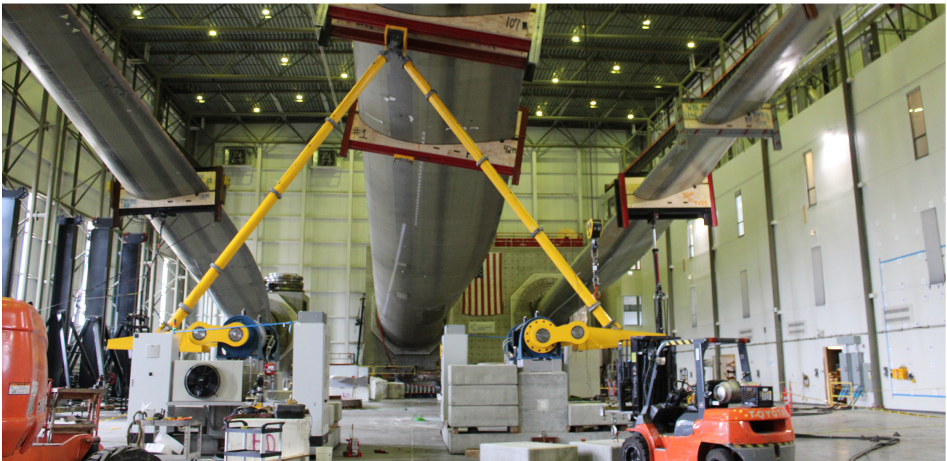
The Massachusetts Clean Energy Center’s Wind Technology Testing Center (WTTTC) offers a full suite of certification tests for utility-scale turbine blades and blade sections. Photo courtesy of WTTTC.
