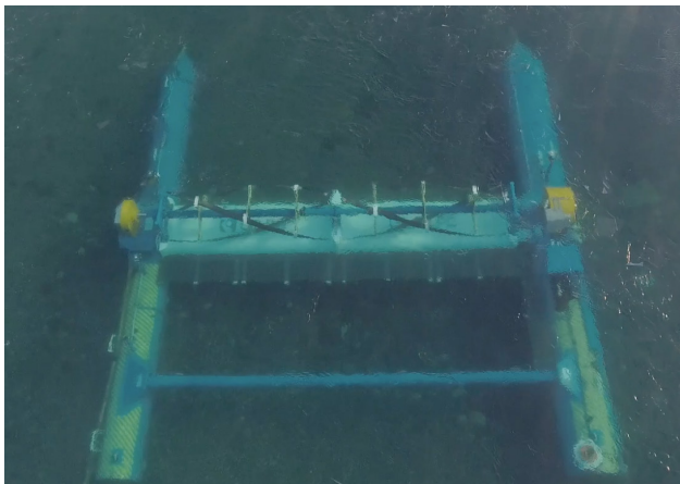
ORPC's RivGen 2.0 deployed in Igiugig, Alaska, to harness energy from the free-flowing current of Kvichak River. Photo courtesy of ORPC
