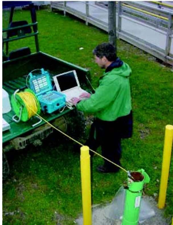
Using a Datalogger to Record Hydraulic Conductivity Data From an On-Site Monitoring Well
