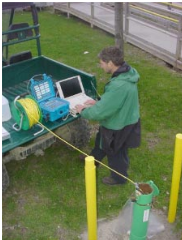
Using a Datalogger to Record Hydraulic Conductivity Data From an On-Site Monitoring Well
