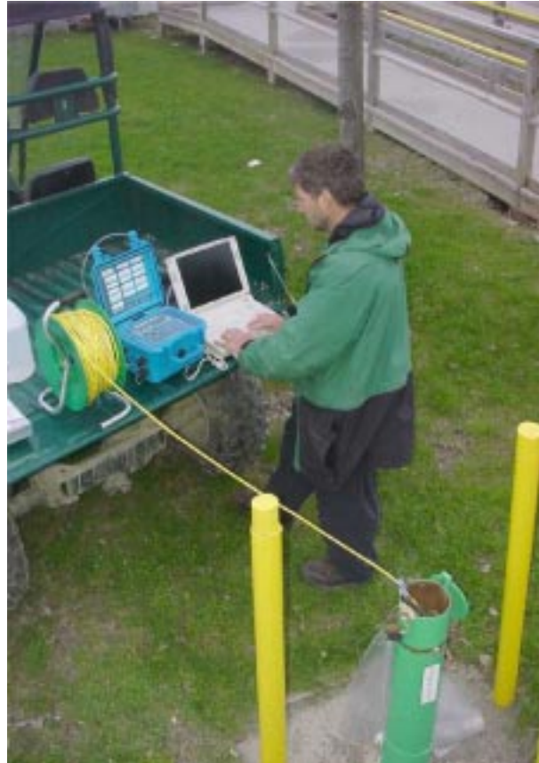
Using a Datalogger to Record Hydraulic Conductivity Data from an On-site Monitoring Well
