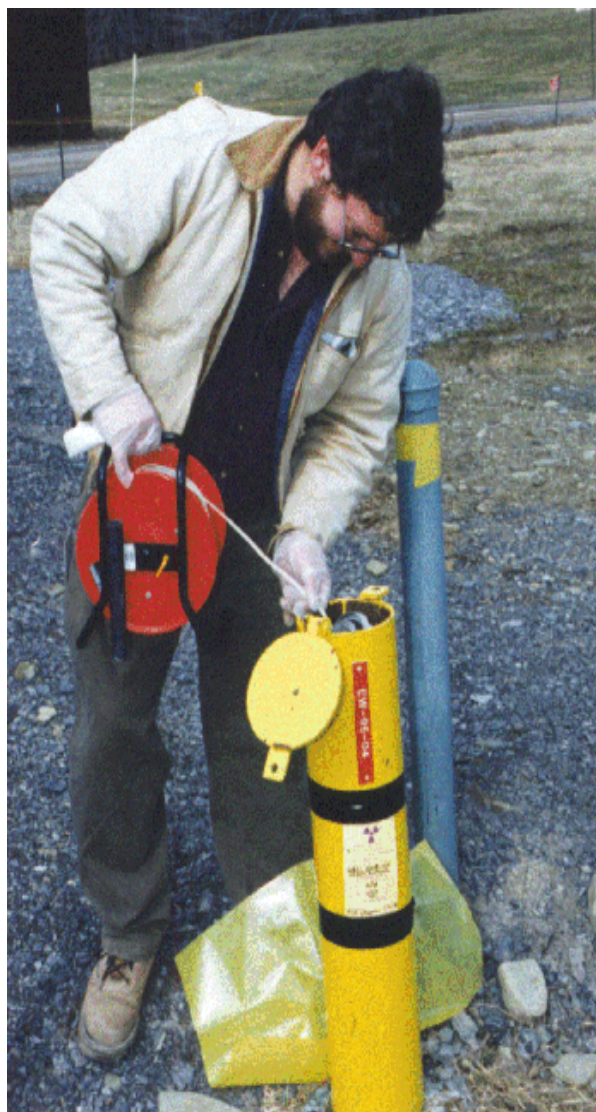
Measuring Water Levels in a Groundwater Monitoring Well
