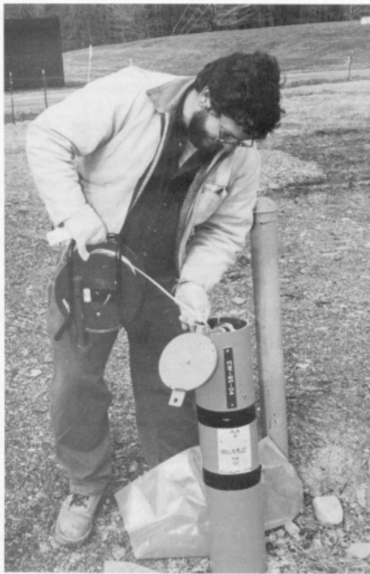
Measuring Water Levels in a Groundwater Monitoring Well
