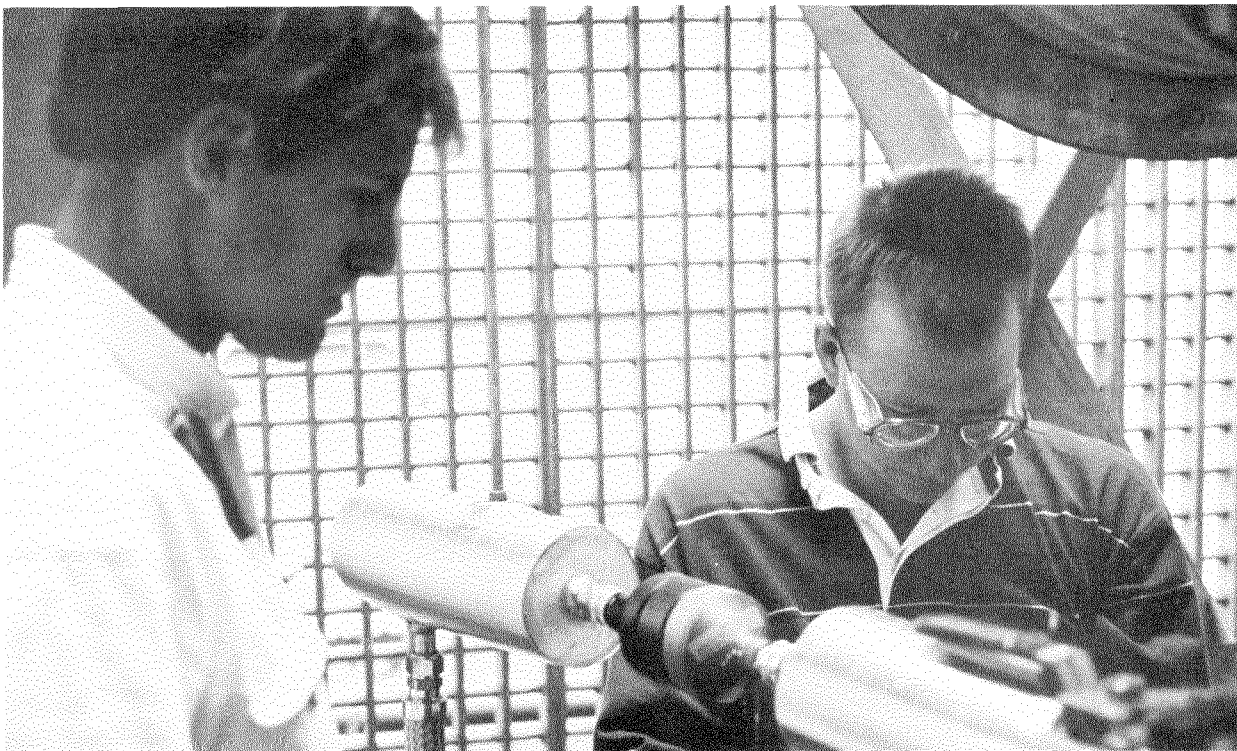
Collecting Baseline Air Effluent Samples from the Vitrification Facility
