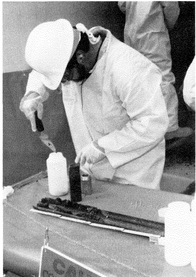
Collecting a Soil Core Sample for Analysis
