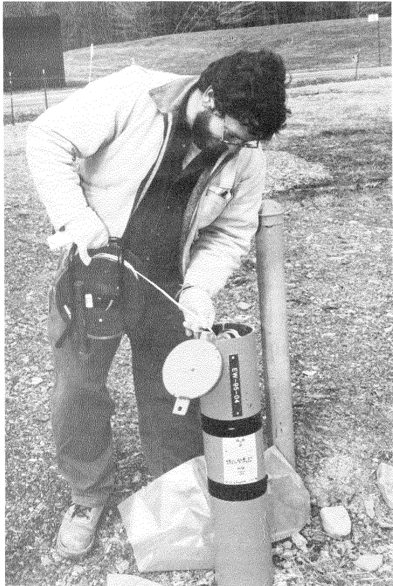
Measuring Water Levels in a Groundwater Monitoring Well
