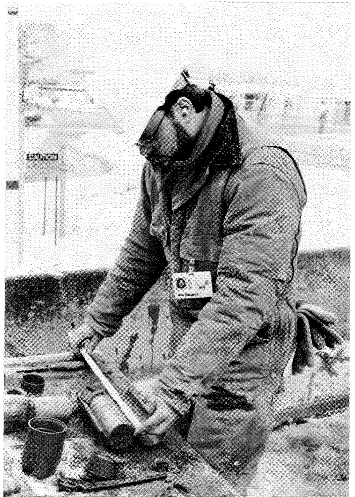
Measuring a Soil Core Sample
