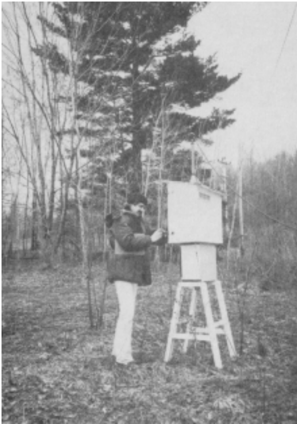
Servicing a Perimeter Air Sampler
