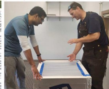
NREL scientists Dr. Ravi Kishore and Dr. Chuck Booten construct "ice boxes" that contain thermal storage ceiling tiles.
