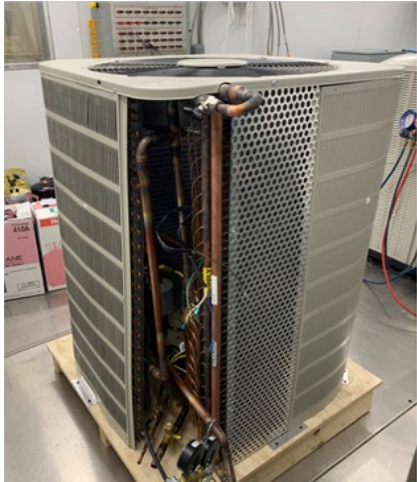
10 Outdoor 5 mm tube coil installed on 4.5 ton chasis
