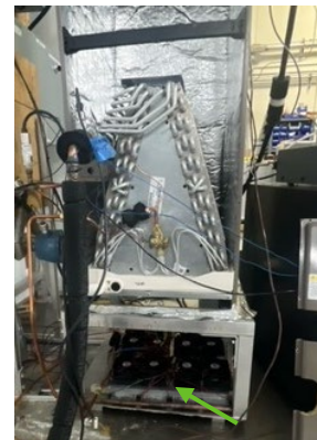
Integration of refrigerant-to-air TE HP
