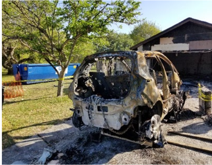
Figure I.32.2 Electric Vehicle and Energy Storage System after burn test
