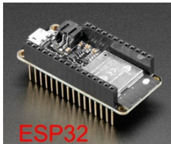
Figure I.5.1 An example of the ESP32 microprocess developed for installation inside a dispenser
