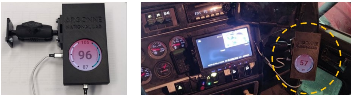
Figure I.6.7 Left - 3D printed phone case and phone displaying the fuel gauge. Right - First installation of assembly in a ready-mix concrete truck is highlighted by the yellow dashed circle.
