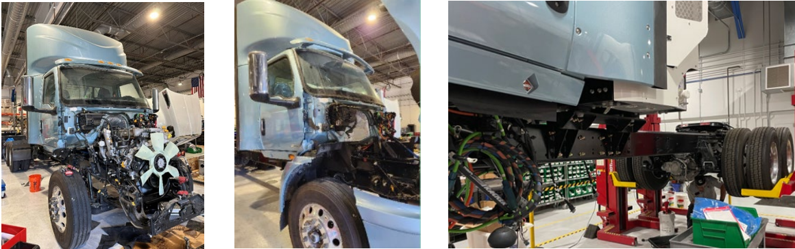
Figure I.16.1 Removal of OEM Parts and eAxle Installation. Source: Cummins Inc
