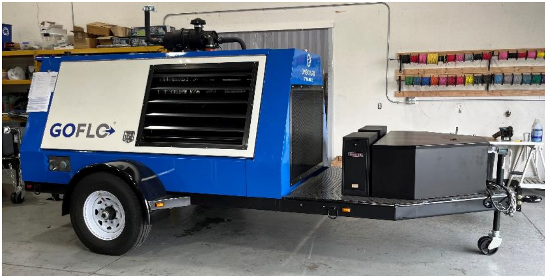
Figure I.38.1 Factory commissioned CNG compressor awaiting shipping from Bend, Oregon
