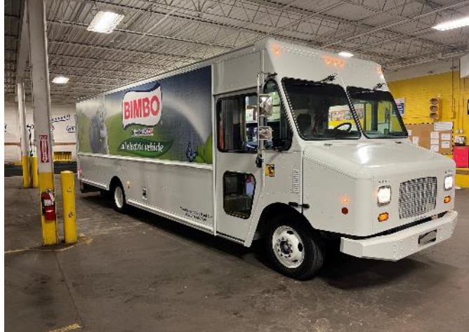
Figure I.22.2 Bimbo Bakeries Class 6 Motiv Power Systems EV Delivery Van in Dayton, OH
