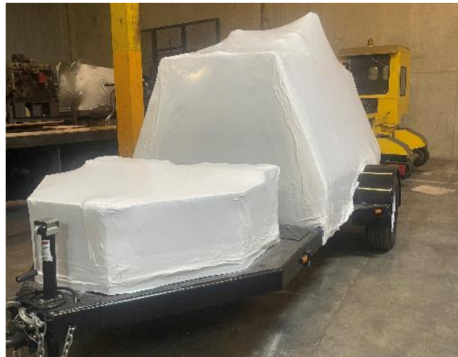
Figure I.38.3 Shrink wrapped compressor awaiting barge shipping to Anchorage, Alaska
