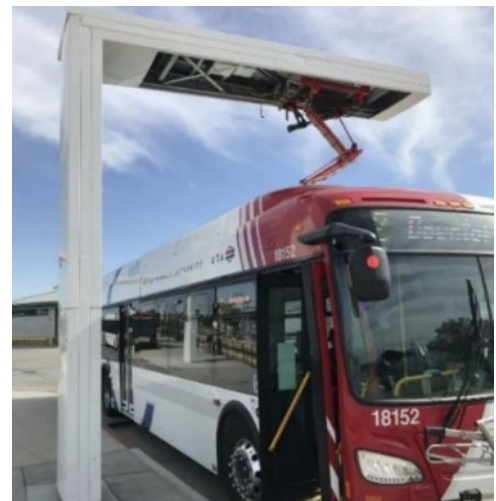
Figure I.26.4 Traction Power Substation (left) and Overhead bus charger (right) (Photo: Utah Transit Authority)
