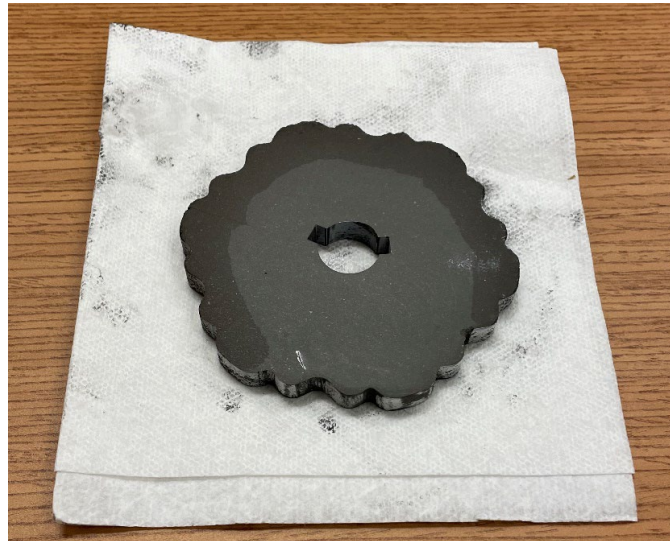
Figure I.1.11.9 DHAM rotor after complete demolding and polishing. A hairline fracture, barely visible in the image, is the only defect in this sample.
