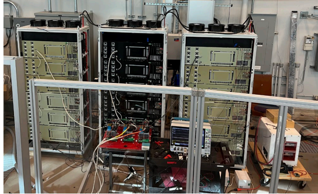
Figure II.1.13.2 Prototype of one phase of the SST assembled in the lab with the front panels in place.
