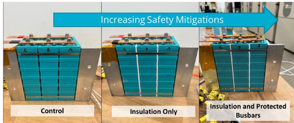
Figure II.4.2.10 Three different thermal control strategies were used for three 20 Ahr lithium iron phosphate cells connected in parallel.
