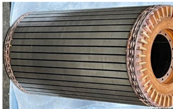
Figure I.2.4.6 Assembled induction rotor with non-insulated copper bars (left) and insulated copper bars (right)
