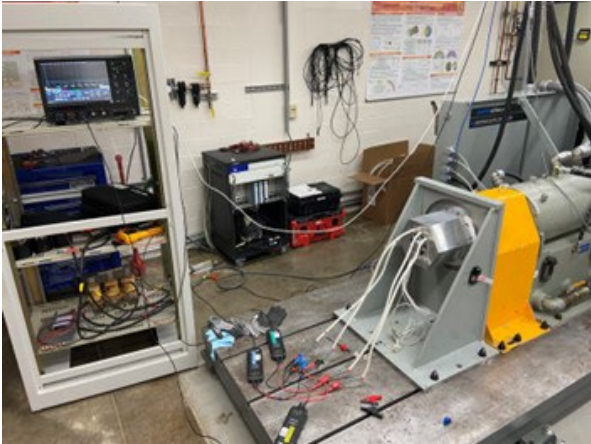
Figure I.1.17.6 Dynamometer test configuration for back-EMF measurement
