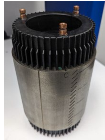
Figure I.2.4.9 Injection over molded stator assembly using CoolPoly D5110
