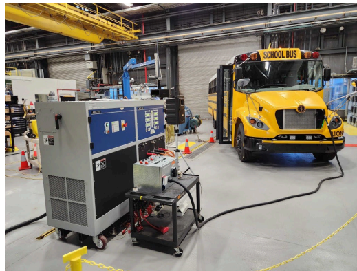
Figure II.3.1.8 Demonstrating a V2G session with the Lion Electric Bus at ANL.
