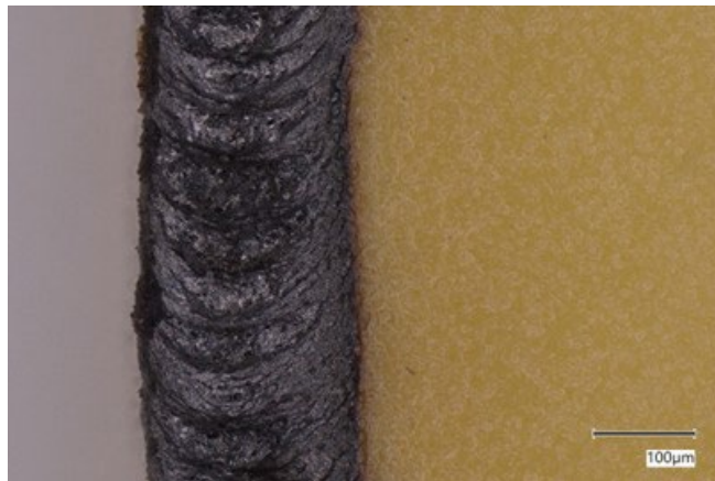
Figure I.1.6.6 HAZ from 30-W, 10.6- \mu\text{m} CO 2 desktop laser cutter
