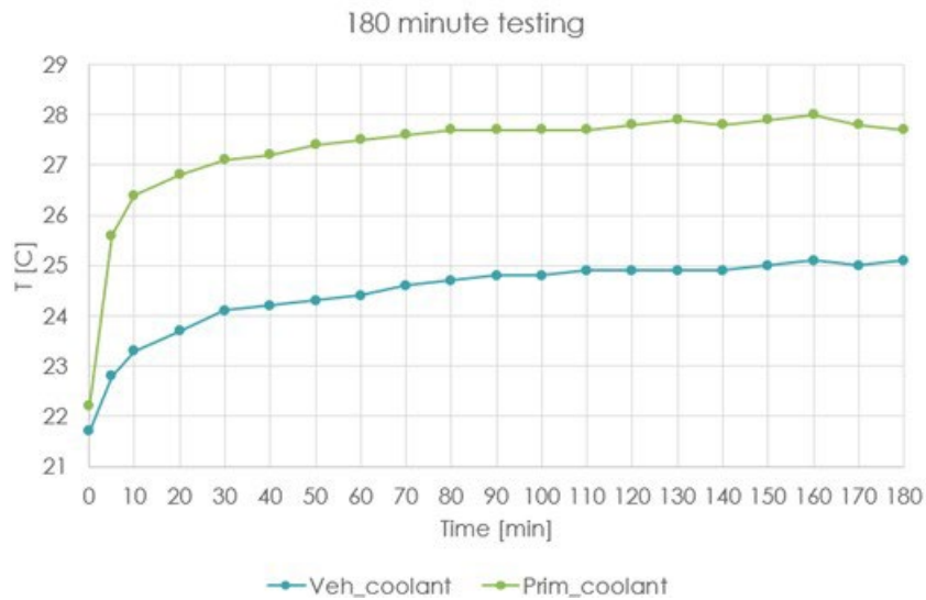
Figure II.1.8.5 Temperature profiles of the primary-side and vehicle-side coolant for a three-hour charge duration.
