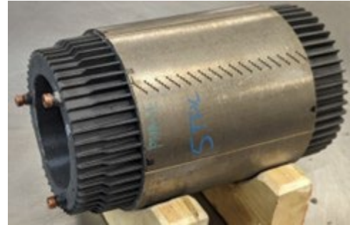
Figure I.2.4.8 Potted stator assembly using EP-3500 material
