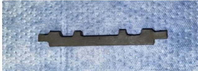
Figure 7. 50% scale version of the DHAM short stator assembly. This component consists of 55 vol.% Fe 4 N.
