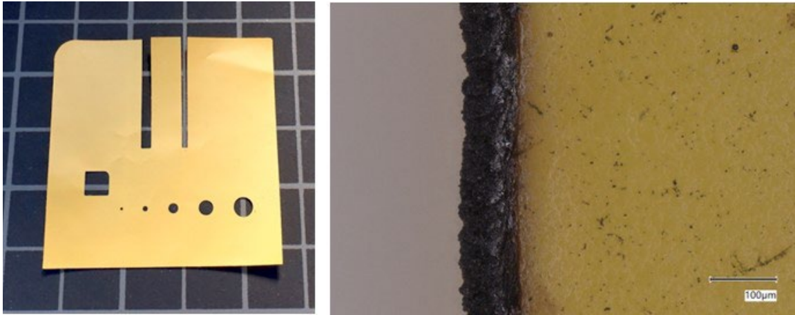
Figure I.1.6.3 Test pattern and HAZ before ultrasonic cleaning
