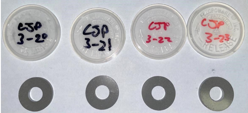
Figure I.1.11.2 Soft magnetic toroids with an Outer Diameter (O.D.) of 35 mm.
