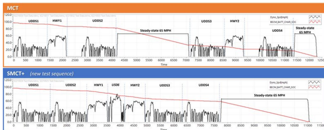
Figure II.6.1.1 Test sequence diagrams for the MCT (from older version of J1634) and the SMCT+ (from latest version of J1634)
