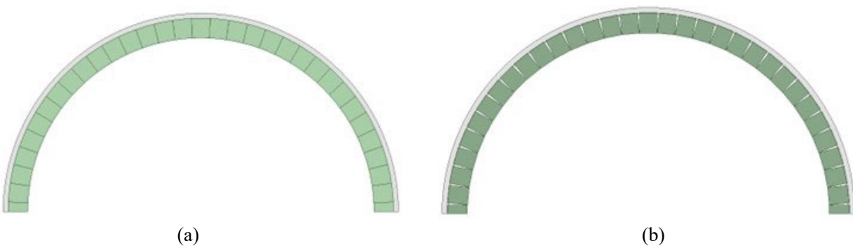
Figure I.1.1.3 (a) Original and (b) modified rotors. The arc magnets were flattened, and locating tabs were included in the rotor core.
