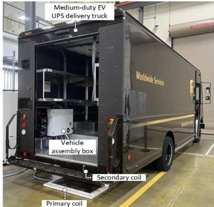
Figure II.1.8.3 UPS truck with bidirectional wireless charging with full operation at the ORNL's GRIDC facility.
