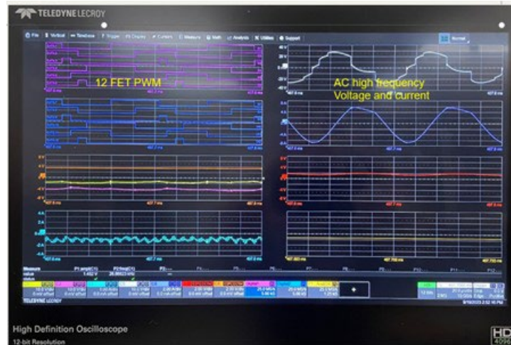
Figure II.1.9.4 Successful modulation generation on AC-AC convertor
