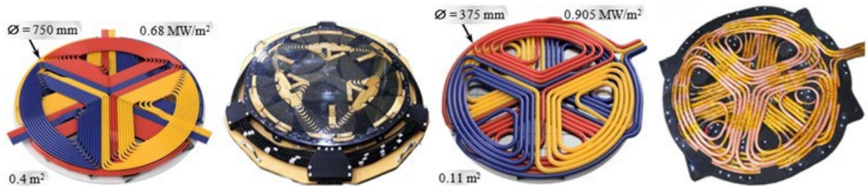
Figure II.1.1.3 Transmitter and receiver coil diameters, geometric designs, and surface power density.
