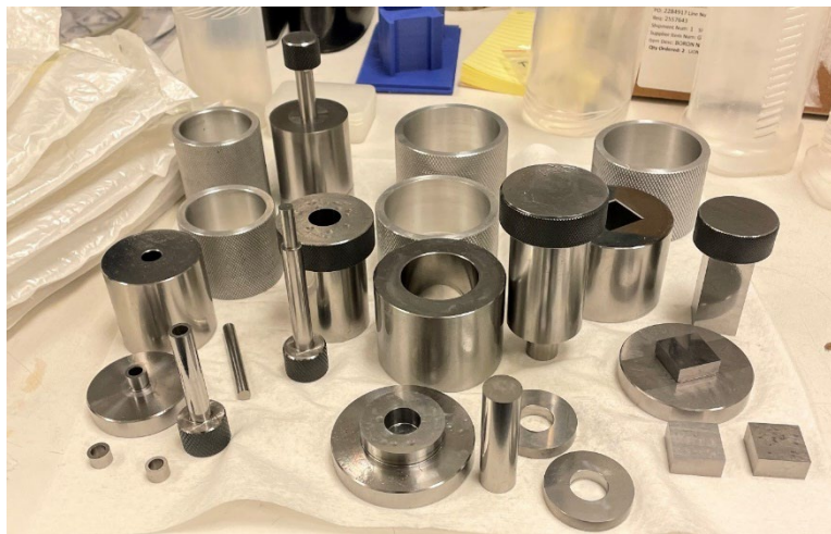
Figure I.1.11.1 Die for pressing larger toroids and cubes.
