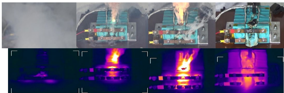
Figure II.4.2.11 Nail penetration of the insulation only module.
