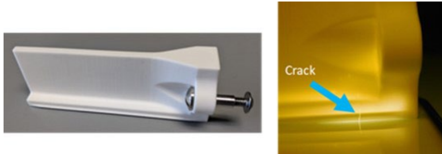
Figure I.1.10.3 Ceramic T-shape in-slot heat exchanger 3D-printed by Lithoz from alumina (left) and crack after sintering (right). Illustration by Bidzina Kekelia, NREL
