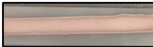
Figure I.1.16.4 Typical copper conductive ink printed on AlN.
