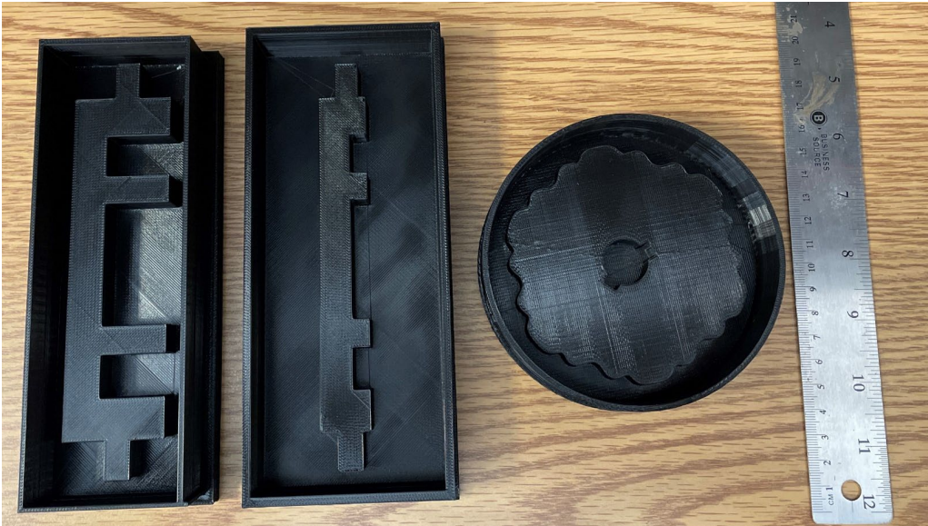
Figure I.1.11.3 PLA anti-molds for the fabrication of DHAM soft magnetic components. From left to right: stator long leg assembly, stator short leg assembly, and rotor assembly.
