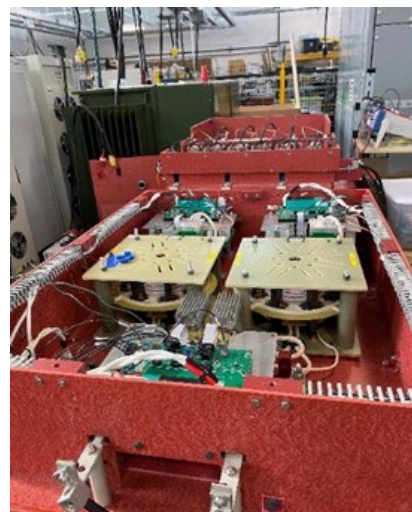
Figure II.1.2.7 DC-DC Module and Unfolder after assembly
