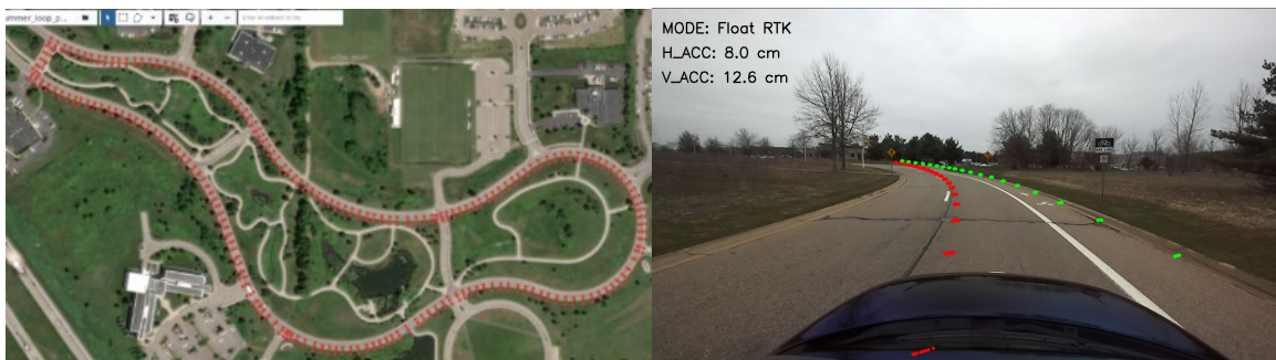
Figure II.1.11.4 projected GPS points from the HD map from a saved OSM file
