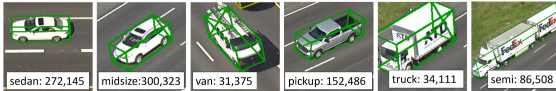
Figure II.1.1.2 Vehicle classification performed by I-24 MOTION permits application of the most appropriate energy models [10]
