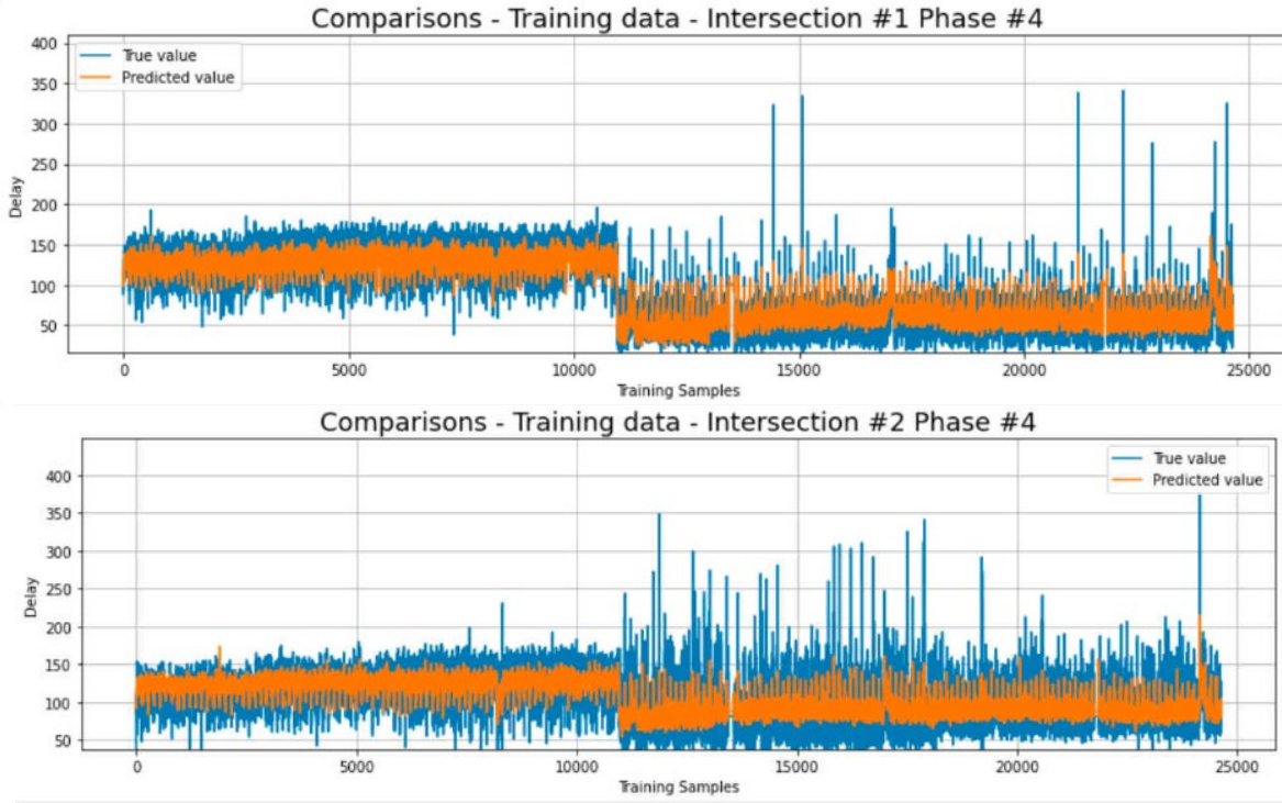
Figure I.3.3.6 : Comparison of actual versus predicted values for some intersections in Corridor #1
