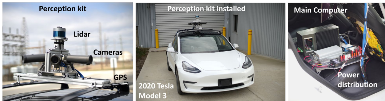
Figure I.1.4.2 At left: Perception system including LiDAR and 6-camera array, at center: system mounted on test vehicle, at right: purpose-built perception computer with neural network object detection and sensor fusion in real-time
