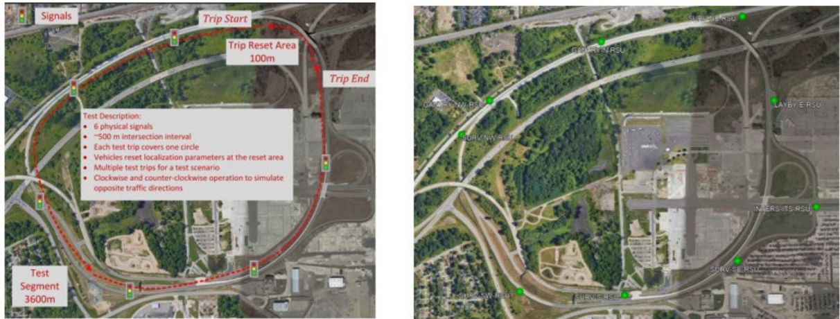
Figure I.4.2.2 Left: ACM test track to be used for intersection traffic signal tests: six traffic signal locations; Right: ACM facility: locations of traffic control cabinets (green dots)
