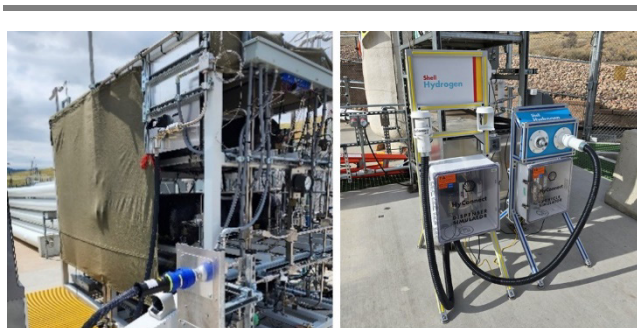
Figure 1. Heavy-duty vehicle simulator tank array (left) and dispenser communication module (right)
