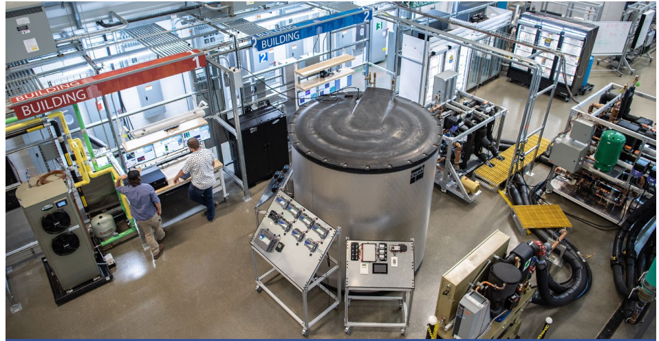
Figure 2. Commercial buildings labs emulate the grid and environment with real building equipment and the ability to switch to any building or location.
