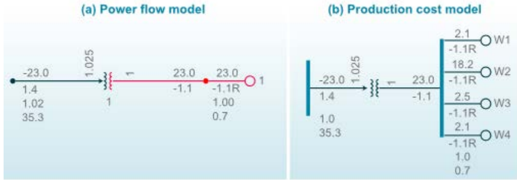
Figure A-2. Generators modeled as one lumped unit versus several distributed units at the same bus in the (a) power flow and (b) production cost models
