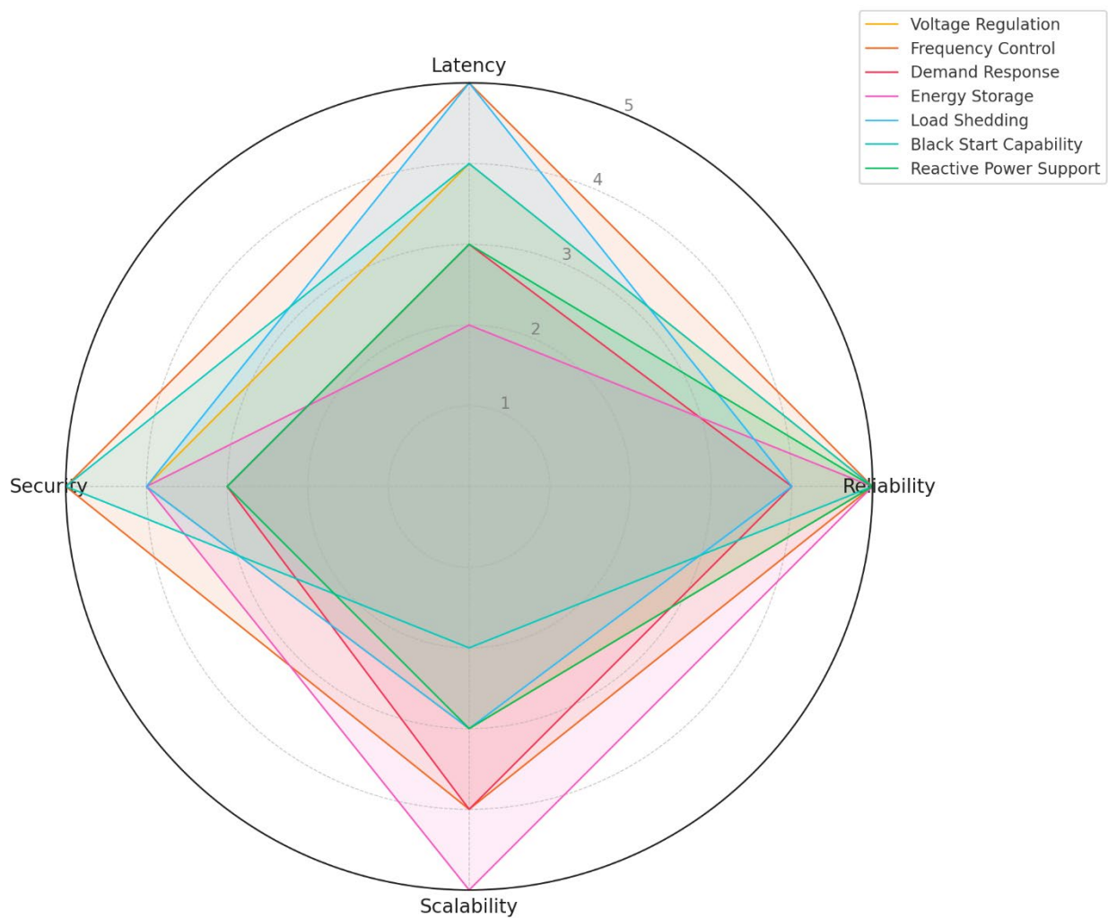
Figure 4. A visualization of the requirements (scale 1 to 5) for some key grid services.
