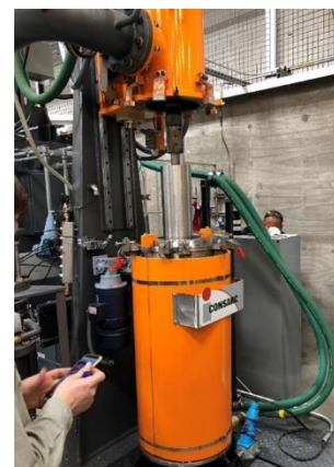
The Development Vacuum Arc Remelt Furnace at the Testing and Development Facility
