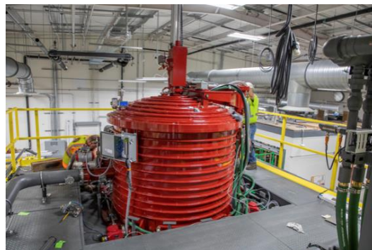
The Multi-Zone Direct Cast Vacuum Induction Melt Furnace
