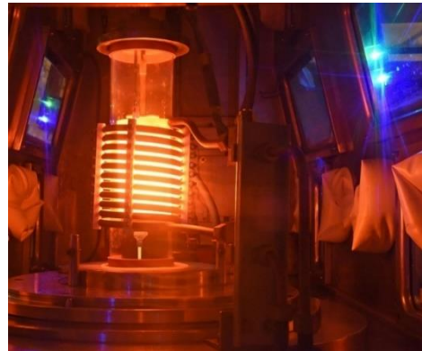
A vacuum induction furnace safely melts and casts plutonium metal, a part of the pit production process at Los Alamos National Laboratory.
