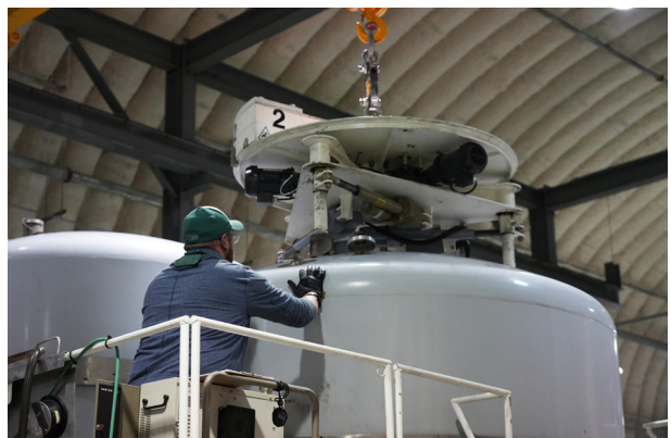
Workers load processed TRU waste into a shipping cask
