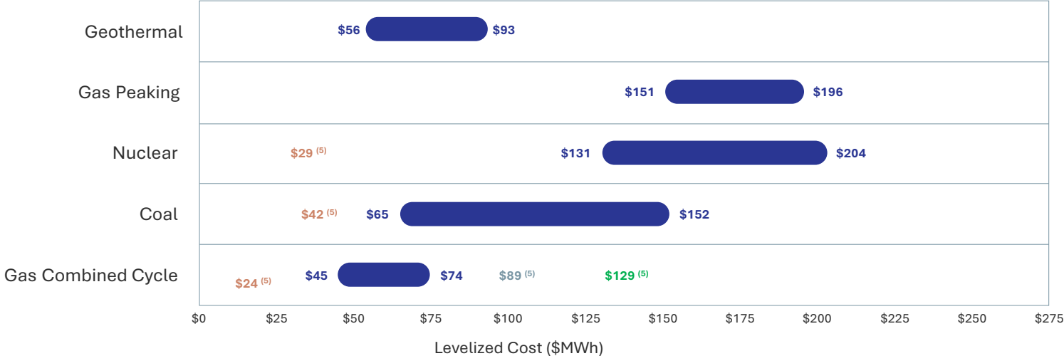
Levelized Cost of Energy Comparison—Unsubsidized Analysis
