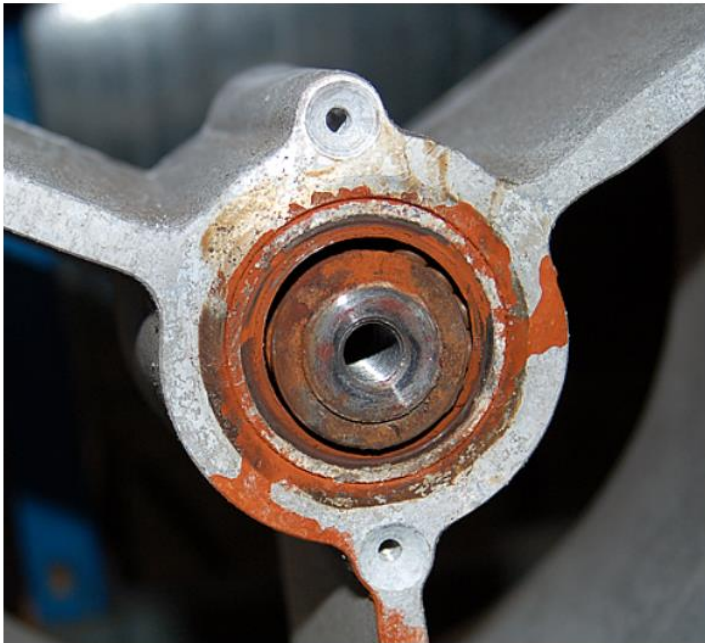
Wheel with Permanently Lubricated Bearing in the Outside Airstream
