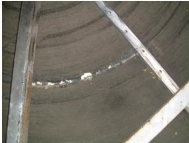
Wheel Damaged by Spoke Deflection
