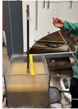
Figure 18: Foundation Load Testing
