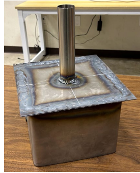
Figure 14: Bucket Foundation Prototype
