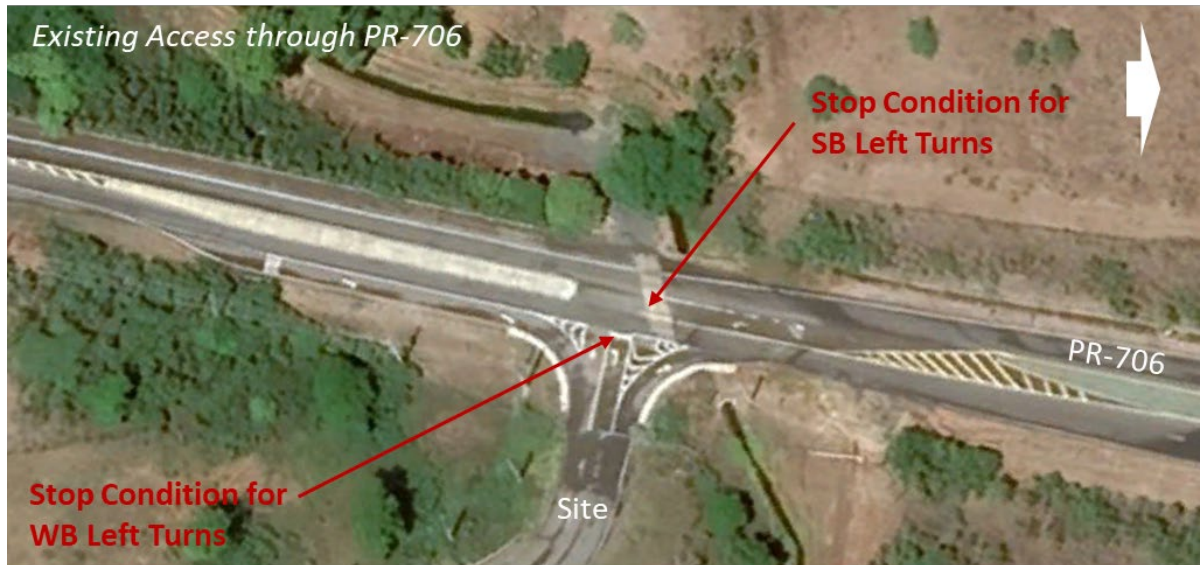
Figure 8 Traffic Control of the Access through PR-706 (Intersection 3)
