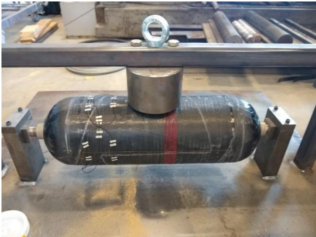
Heavy Impact Test Set Up
