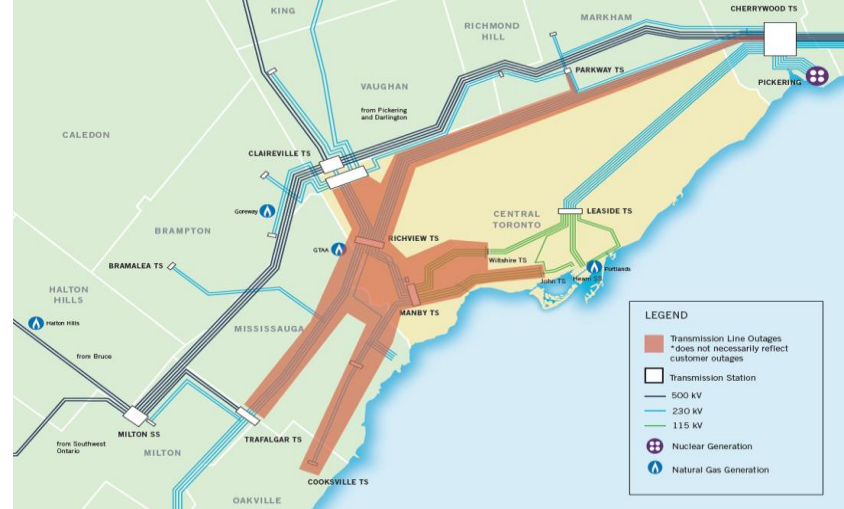
The flooding resulted in the loss of 25 230kV circuits and 4000MW of load
