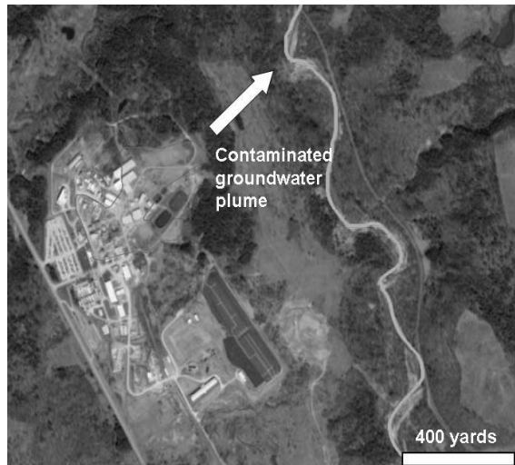
Figure 3.3 The Groundwater Plume Contaminated with Strontium-90 (indicated in green) is Migrating Towards Buttermilk Creek (indicated in blue) 13
