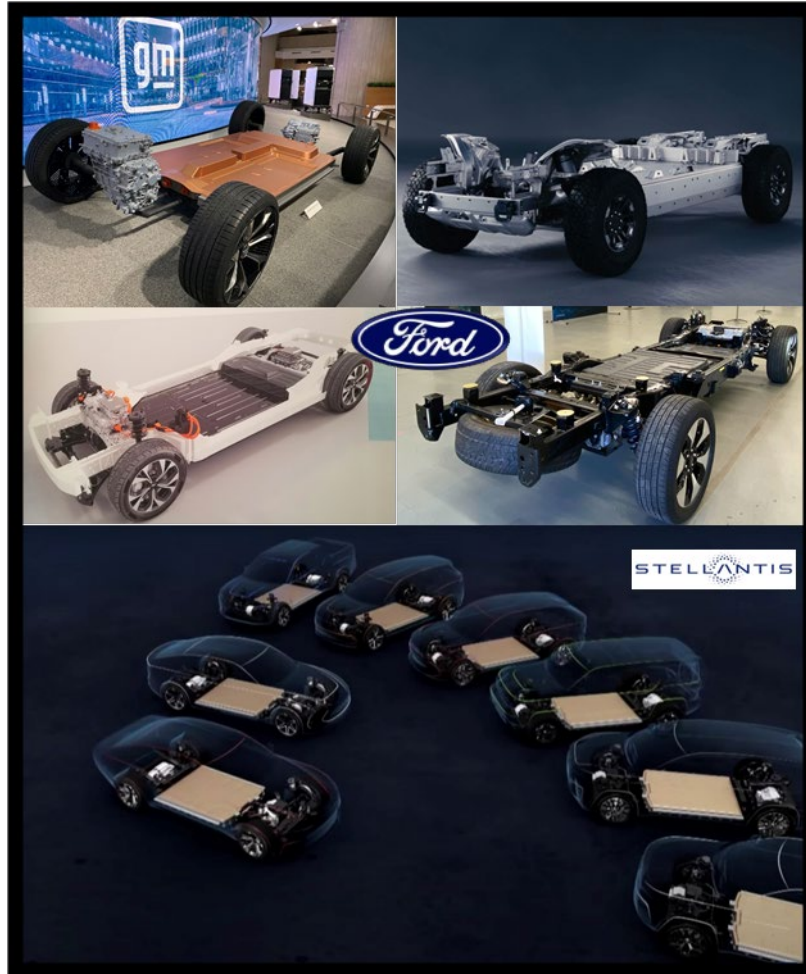
Figure 10. Examples of Skateboard Chassis Containing Electric Powertrain for passenger and trucks.
