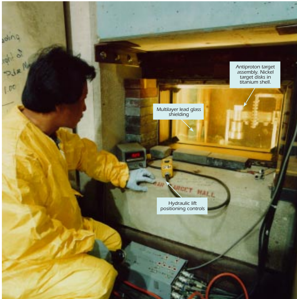
Exhibit 4-5: Technician observes hot target from behind lead glass shielding.
