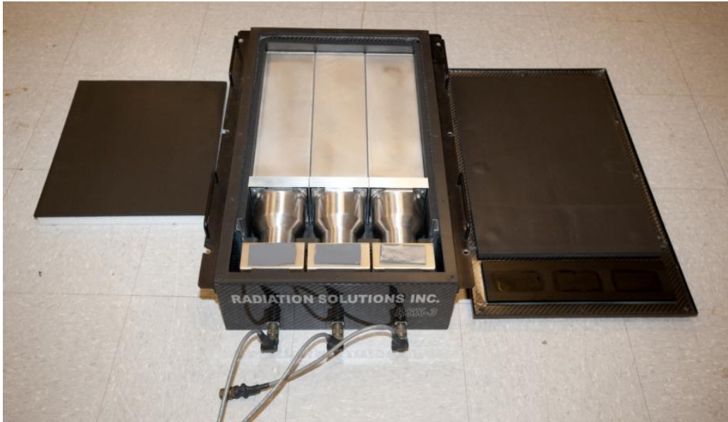
Figure 2: RSX-3 detector unit with three 2" × 4" × 16" NaI(Tl) scintillators, three photomultiplier tubes, and three ADS modules.
