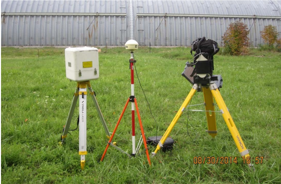
Figure 5: Gamma in situ measurement using ionization chamber, GPS antenna, and high-purity germanium spectrometer.
